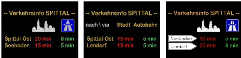
Fig. 2. Design alternatives of the category “ schedule oriented ”. On the left the design with text (VMT), in the middle with icons (VMI) and on the right with icons and signposts (VMW).
