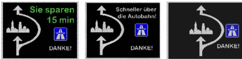
Fig. 3. Design alternatives of the third category “ icon oriented ”. On the left an alternative with additional information on the saved time (“ You save 15 minutes / Thank you! ”) (UMZ), in the middle an alternative with a general hint (“ You are faster via the by-pass / Thank you! ”), (UMT), on the right just the symbol with an icon and “ Thank you! ” (UOT).
